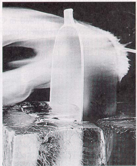
FIGURE 1-9 Cookware made of a glass-ceramic provides good mechanical and thermal properties. The casserole dish can withstand the thermal shock of simultaneous high temperature (the torch flame) and low temperature (the block of ice). (Courtesy of Corning Glass Works)
