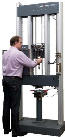
**Figura 41 - Drop Weight Tester HIT230F**
